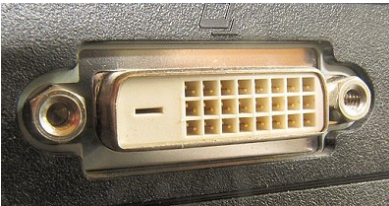
DVI-D-Anschluss (Digital Visual Interface) DVI-D-Kabel (Dual-Link) haben 24 + 1 Pins.
